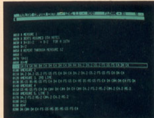
Notes may be entered in from the Music Keyboard directly and timing information can be added later using the Editor Controls on the Alpha-numeric keyboard. Line numbering (left hand column) is provided automatically.
