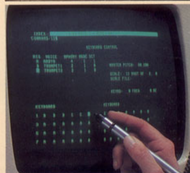
KEYBOARD CONTROL: Provides allocation of Voices to various Registers in the keyboard or sequencer. In this example ANDY8 is able to play 4 note polyphonically in register A which is on all keyboards except for keyboard 1, where the top 3 octaves are playing "TRUMPET2" (Register C) and the bottom 3 octaves are playing "TRUMPET1" (Register B). Selection of keyboard registers is done with the light-pen. The top right hand page allows pitch adjustment and scale changing.
