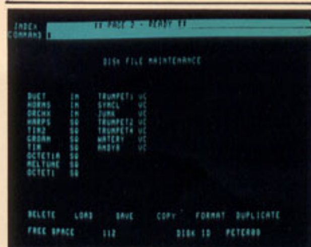
DISK FILE MAINTENANCE: Displays the names of "files" which are available for loading from the user's disc. Files may describe Voices (the sounds themselves), Sequences, and Instruments (combinations of sounds with control details). Other special files such as composition sequences can be accessed via this page, operating the light-pen enables loading of sounds from the disc in several seconds.
